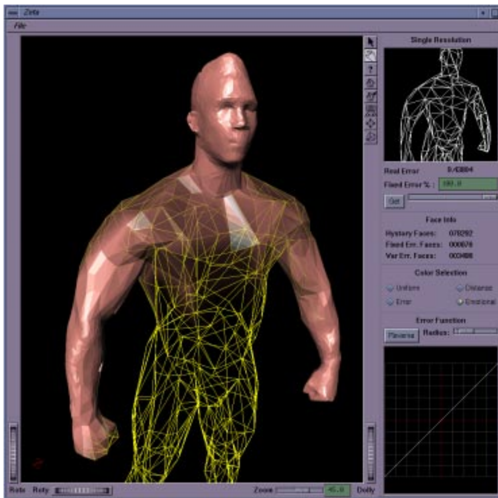
Figure 30: The interface of Zeta, a resolution modeling prototypical system; the resolution modeling session started on a low resolution representation of a mesh distributed by Cyberware Inc. (the GMM model consists of 78k facets); then we selectively refined it (few composed refinement actions were operated in the areas of the head and the arms).
