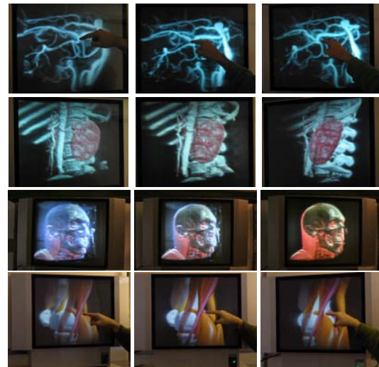
Figure 3: Real-time inspection of medical volumetric models visualized with a lightfield display [AGI*08]. Pictures are taken with an hand-held camera at different viewing angles, in order to highlight the horizontal parallax of the light field display.
