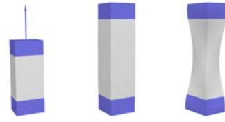
Figure 13: Illustration of the effect of the different shape modeling constraints. Left: handle constraints are specified to fix the bottom of the box and to move the top to the desired position. Middle: with only the rigidity constraint the total volume is increased by 53%. Right: the total volume remains within 3% of the original when the volume constraint is added.
