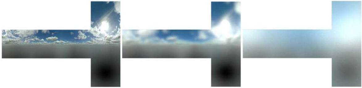
Figure 8.6: Examples of filtered environment maps: Original environment map ( left ). Filtered version with a specular exponent s = 100 ( middle ). Irradiance map created by filtering over the entire hemisphere ( right ). (Shader code in Listing 8.1)
