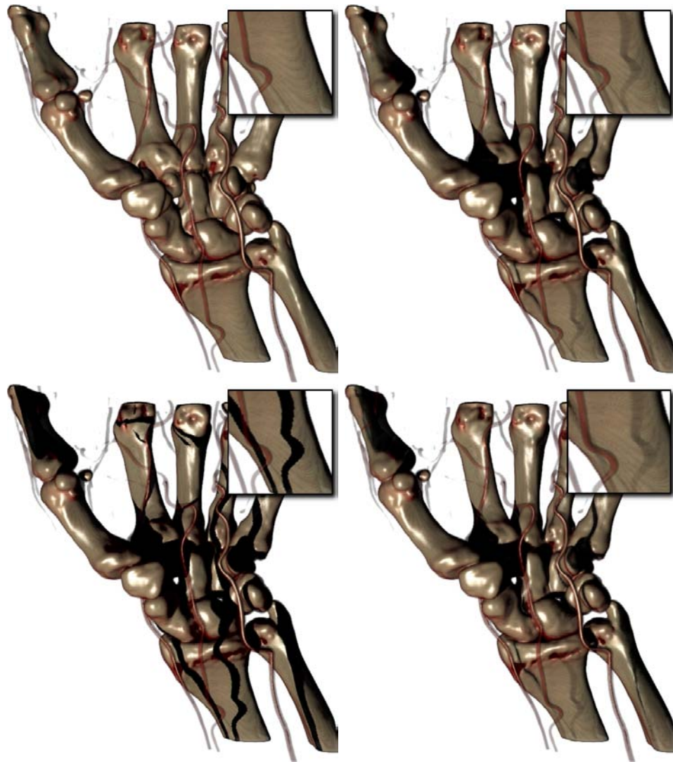
Figure 4.8: The hand data set ( 244 \times 124 \times 257 voxel) rendered without shadows, with shadow rays, with shadow mapping and with deep shadow maps (from top left to bottom right). Semi-transparent shadows become visible when using shadow rays or deep shadow maps.
