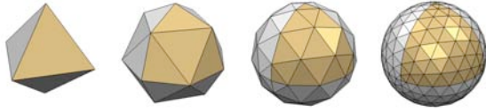
Figure 2: Each subdivision step halves the edge lengths, increases the number of faces by a factor of 4, and reduces the error by a factor of \frac{1}{4} .
