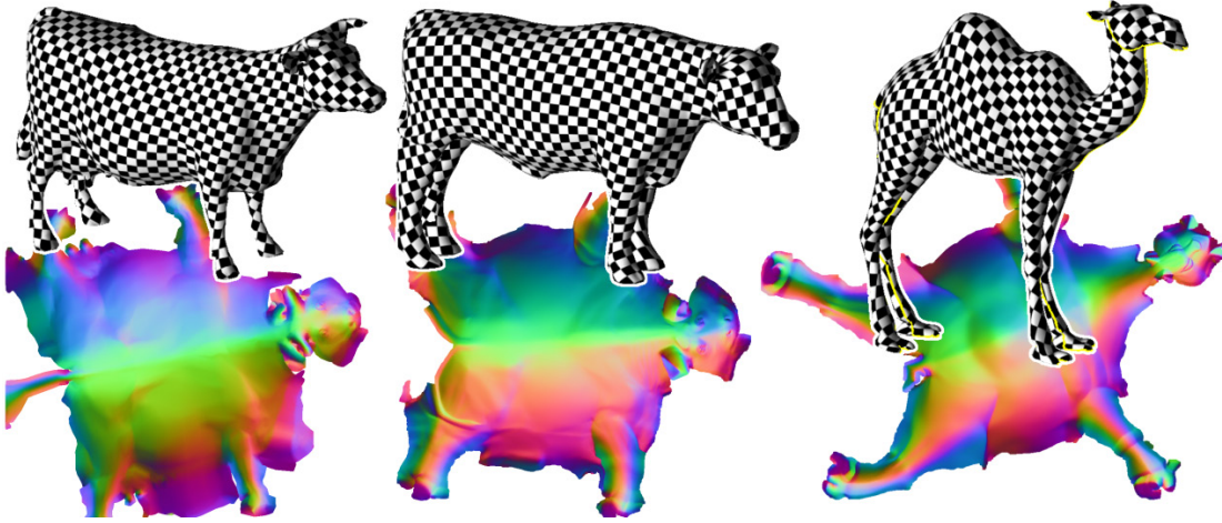
Figure 8.13: Some results computed by stretch L_2 minimization (parameterized models courtesy of Pedro Sander and Alla Sheffer).
