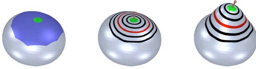
Figure 11.2: After specifying the blue support region and the green handle regions ( left ), a smooth scalar field is constructed that is 1 at the handle and 0 outside the support ( center ). This scalar field is used to propagate and damp the handle’s transformation ( right ).
