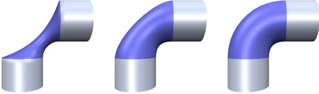
Figure 7.6: The order k of the energy functional and of the corresponding Euler-Lagrange PDE \Delta_S^k \mathbf{x} = 0 defines the stiffness of the surface in the support region and the maximum smoothness C^{k-1} of the boundary conditions. From left to right: membrane surface ( k = 1 ), thin-plate surface ( k = 2 ), minimum variation surface ( k = 3 ).
