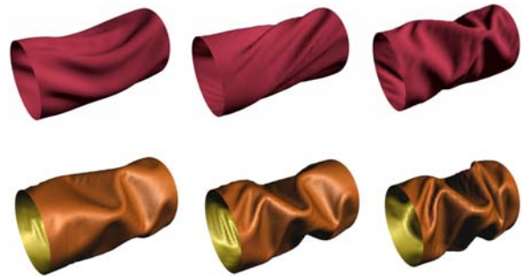
Figure 15: Top: Different types of folds on a garment's sleeve generated using a typical textile material. Bottom: Sequence taken from an animation of axial compression of a cylinder with a metal-like material.
