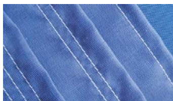
Figure 19: Effect of seam pucker
