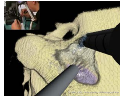
Figure 31: Snapshot taken from IERAPSI surgical system, where a ENT trainee is performing a mastoidectomy. The inset shows the hardware setup, composed by two PHANToM haptic interfaces and a NVision binocular display
