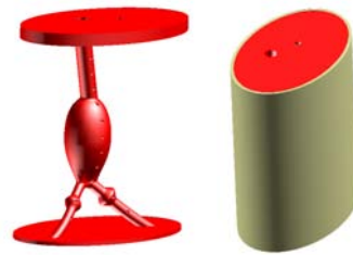
Figure 38: Aneurysm phantom realized at University of Innsbruck and used to validate the aortic measurement system.
