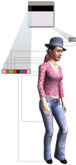
Figure 24: A CLUT image used to store the color of each virtual human body parts and accessories.
