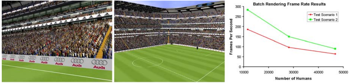
Figure 16: (a) Rendering thousands of characters in a single draw call. (b) Frame rate results.
