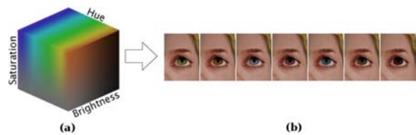
Figure 18: The HSB space is constrained to a three dimensional color space with the following parameters (a): hue from 20 to 250, saturation from 30 to 80 and brightness from 40 to 100. Colors are then randomly chosen inside this space to add variety on the eyes texture of a character (b).
