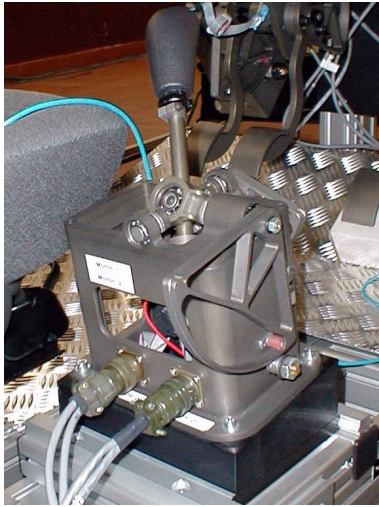
Figure 43: The haptic interface simulating the gearshift
