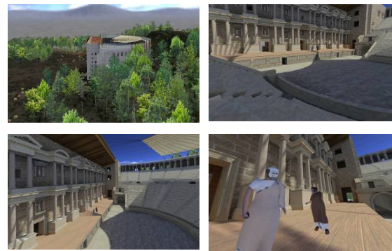
Figure 14: Screenshots from the final 3D interactive real time simulation featuring our adapted Precomputed Radiance Transfer illumination model for deformable characters and a diffuse map-lightmap approach for static surfaces
