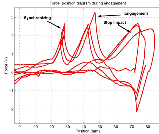
Figure 44: The simulated force response of a gearshift
