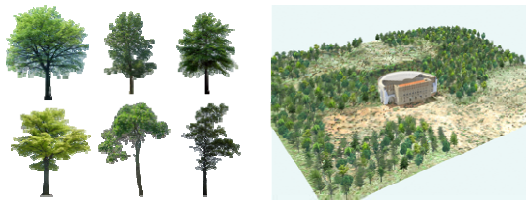
Figure 2: Samples from the billboard collection representing the vegetation (left) and rendering of the final model of the environment of the theatre of Aspendos (right)
