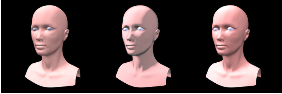
Figure 27: Images generated using the D-O model (left), a Lambertian Model (middle) and the H-K model (right). (Courtesy of Jos Stam).
