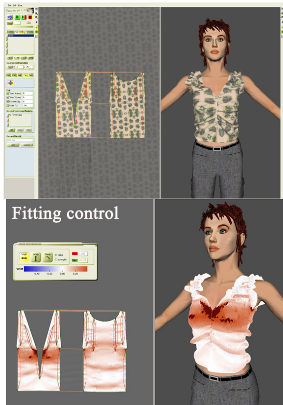
Figure 13: Interactive garment prototyping and comfort evaluation: More than the garment shape and appearance design (left), the system also allows mechanical comfortability data to be evaluated directly with any change of the pattern design and sizing (right).
