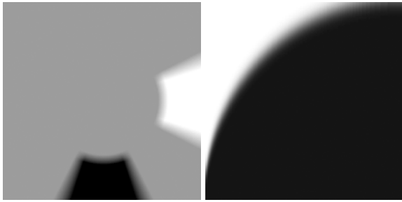
Figure 9: Two-dimensional transfer functions in curvature space. (left) Ridge and valley lines in (\kappa_1, \kappa_2) domain [KWTM03]; (right) contour thickness control [KWTM03].
