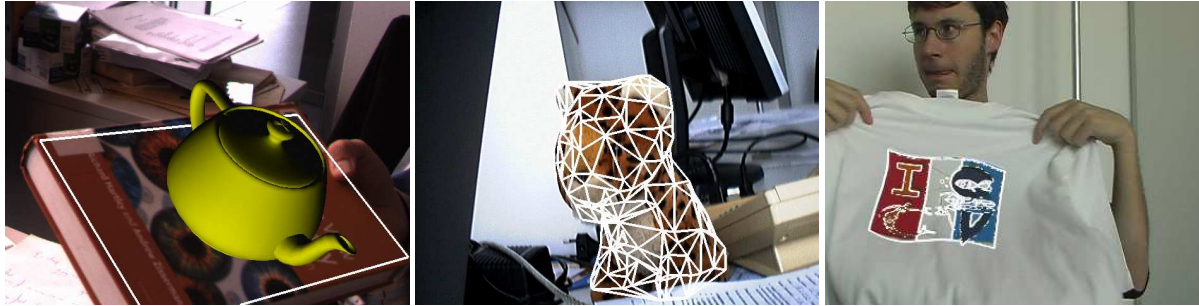
Figure 5: Detection and computation in real-time of the 3D pose of a planar object, a full 3D object, and a deformable object. (From [LLF05] and [PLF05].)
