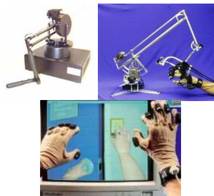
Figure 3. Examples of haptic devices. From the top-left, arm-like device [Pha], exoskeleton [Imm], and tactile display [Imm]
