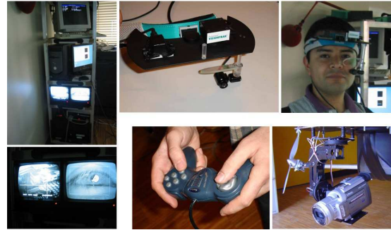
Figure 7: Top and left: The Eye-tracking system. Bottom-right: The mounted rotating camera and the joystick controller.
