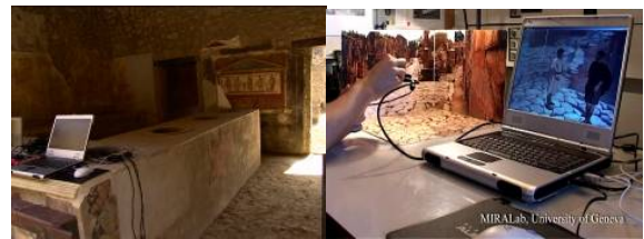
Figure 4 (left). The Real Pompeian ‘thermopolium’ that was augmented with virtual animated virtual characters. In this figure the scene is set-up for camera tracking preprocessing; consequently the laptop is put in the backpack for the run phase. (right) Lab ‘maquette’ controlled AR tests. For optimum flexibility and tests the camera is detached from the HMD and moved freely within the ‘tracked area’ augmenting it with virtual characters (laptop monitor)
