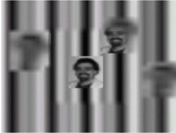
Figure 3: A view presented in the second experiment. Here the periphery uses the 20 x 15 LOD, while the lowest contrast background is used. The central area is (always) displayed at the highest HMD resolution. Four distractors are shown. (Image from [WWH04] courtesy of Ben Watson.)
