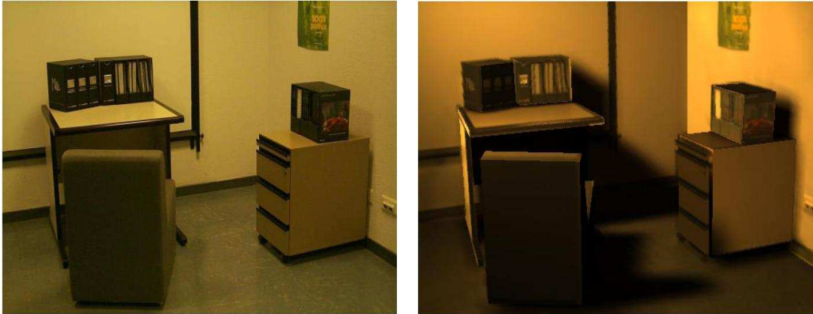
Figure 4: Results for Loscos et al. [LDR00]. The image on the left hand side represents the real scene. The image on the right hand side shows the relighted synthetic scene, for which real light sources have been virtually turned off and a virtual light source is inserted. Global common illumination updates are performed at interactive rates using an adapted version of [DS97]. Courtesy of Loscos et al.
