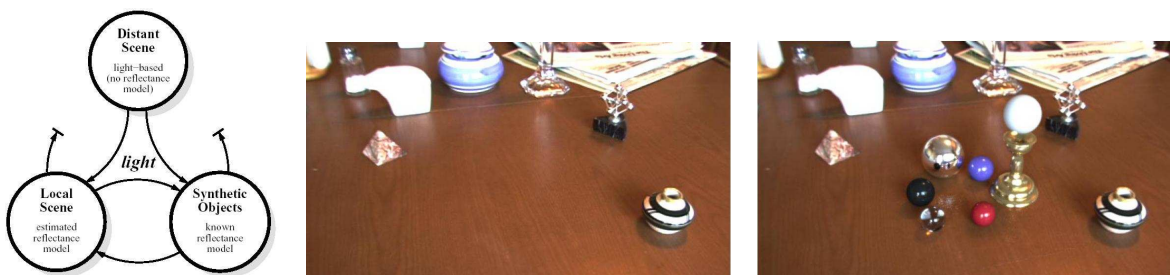
Figure 8: Debevec et al. [Deb98]. Left: a diagram illustrating the relation between the different components presented in [Deb98]. The real scene is divided into a local scene and a distant scene. The illumination from the distant scene influences the local scene and the virtual objects. The virtual objects influence the local scene. The local scene and the virtual objects do not have an influence on the distant scene. Middle: an image of the real scene. Right: an example of the differential rendering technique for an indoor scene after inserting virtual objects. Diffuse effects are simulated. Courtesy of Debevec et al.
