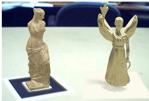
Figure 5: Results for Agusanto et al. [ALCS03]. The virtual objects are rendered with skin textures. The left object is blended with a diffuse map and no soft shadows. The right object is blended with a glossy map and with soft shadows. Courtesy of Agusanto et al.
