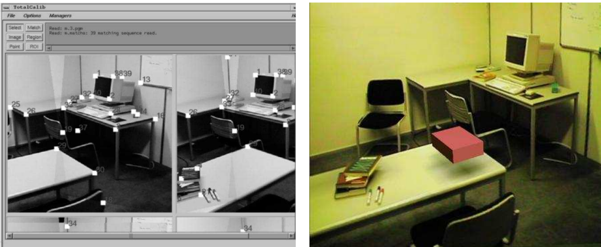
Figure 11: Results for Drettakis et al. [DRB97]. In the left image a screen shot is given of the 3D reconstruction of the real scene. The right image gives an example of the MR, the floating box is the virtual object. The virtual objects can be moved at interactive rate while keeping the global illumination effects. This is carried out by using an adaptation of hierarchical shafts for hierarchical radiosity [DS97]. Courtesy of Drettakis et al.
