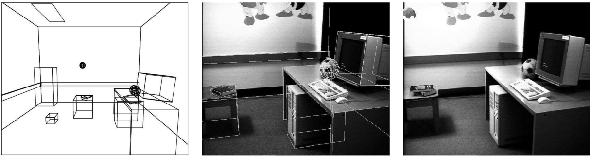
Figure 10: Results for Fournier et al. [FGR93]. Left: wire-frame image, all objects in the scene are represented by a box, that narrowly fits the object. Middle: Image information is mapped on the boxes (not that for the ball, a more complex shape was used). Right: an example of a MR, the book on top of another book, lying on a table is virtual. Also a virtual light source is added. The global common illumination effects are generated with an adaptive progressive radiosity algorithm. Courtesy of Fournier et al.
