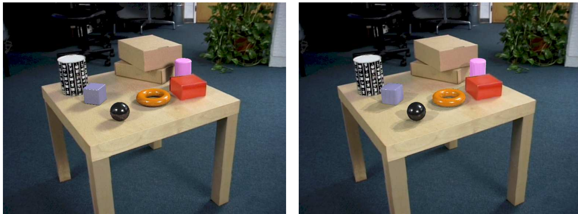
Figure 7: Results for Gibson et al. [GM00]. Comparison of a ray-traced (left) and a hardware generated image (right). The ray-traced image was generated using RADIANCE [War94], the hardware generated image made use of the rendering method described in [GM00]. The generation of the ray-traced image took approximately 2 hours, the generation of the hardware rendered image took place at nearly 10 frames-per-second. Courtesy of Gibson et al.
