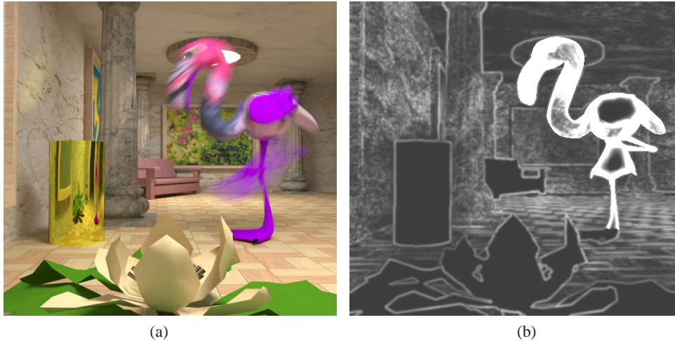
Figure 8: Spatiotemporal error tolerance map processing. (a) An input frame with dynamic objects rendered for a moving camera and (b) the corresponding spatiotemporal error tolerance map obtained using the spatiovelocity CSF processing. Brighter areas on the map denote areas where less effort should be spent in computing the lighting solution. (Images courtesy of Hector Yee, Sumant Pattanaik, and Donald Greenberg.)
