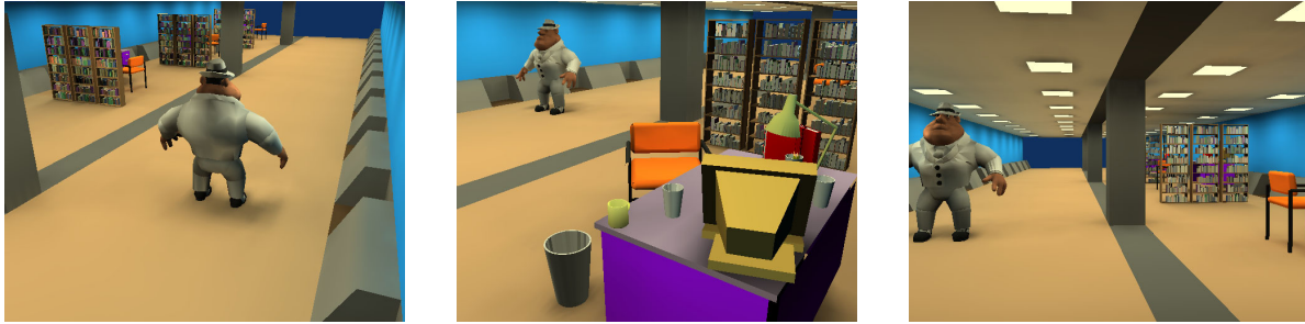
Figure 6: Example stills from a 500 frames long animation computed using Space-Time Hierarchical Radiosity. The scene was build using 35,000 input surfaces. Rendering was approximately 20 times faster than a frame per frame computation, but required 7 times more memory.
