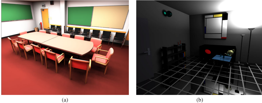
Figure 4: Example frames with global illumination effects obtained using distributed ray-tracing engine for scenes composed of a) 300,000 and b) 34,000 triangles. On a cluster of 16 CPUs (Athlon1800+) the frame rates 1.5 fps. and 1.84 fps. have been achieved, respectively. To fully eliminate all visible image artifacts resulting from changes of the view direction or other changes in the scene 1–2 seconds of the computation are usually required. (Images courtesy of Ingo Wald, Thomas Kollig, Carsten Benthin, Alexander Keller, and Philipp Slusallek.)
