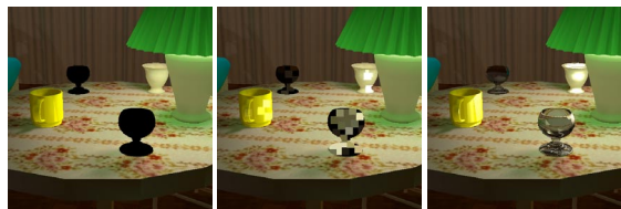
Figure 3: Perceptually Guided Corrective Splating: A rasterized image gets progressively better as more ray traced corrective information is applied. Left: Without corrective information. Middle: After having splat only few corrective samples. Right: Converged image after a few frames.
