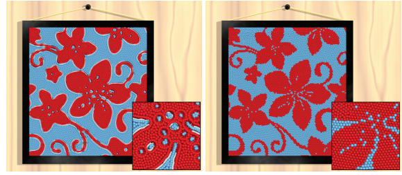
Figure 7: Standard SPH results in spurious behavior introduced by discontinuities across the interface of two fluids with density ratios (left). Adapted equations for multiple fluids according to [SP08] eliminate the artifacts (right).
