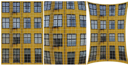
Figure 3: This figure demonstrates the effect of barrel (middle) and pincushion (right) distortions on an image. In this case, the distortions are exaggerated and overlaid with a grid for demonstration purposes. The undistorted image is shown left.
