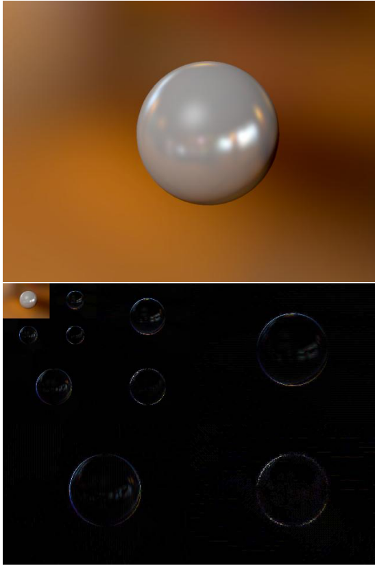
Figure 15: Top: Original image. Bottom: An example of a Haar wavelet decomposition with three scales. The top left image in the decomposition represents averages, whereas the remaining panels indicate differences in horizontal, vertical and diagonal directions.
