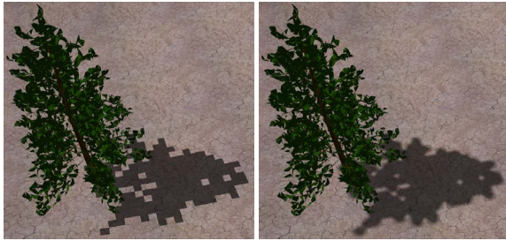
Figure 22: Undersampled unfiltered shadow maps on the left suffer from hard jagged edges. These can be removed by filtering. On the right hardware PCF with a 2 \times 2 kernel is applied.
