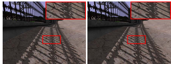
Figure 19: LiSPSM gives good results for a shadow map resolution of 1024^2 and a viewport of 1680 \times 1050 , but temporal reprojection can still give superior results because it is not limited by the shadow map resolution.
