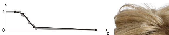
Figure 24: Deep shadow maps store a piecewise linear representation of the transmittance function gathered from various samples at every texel (left). This allows shadow mapping of challenging cases like hair (right).
