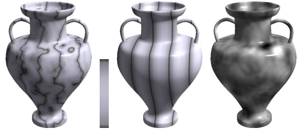
Figure 8: Procedural texture creation. The marble vase (left) is obtained from two components: A color map repeated along the x direction in space (middle), perturbed by a solid noise (right). The final color is obtained as C(x+N(x,y,z)) where C is the 1D color map, N the noise and x,y,z the surface point coordinates. (Figure based on [LLDD09a], ©ACM, 2009.)
