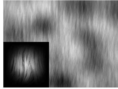
Figure 4: Sparse convolution noise. Lower left: windowed sample from an image of hair. Right: approximate “hair” texture created using 2D sparse convolution using this kernel.
