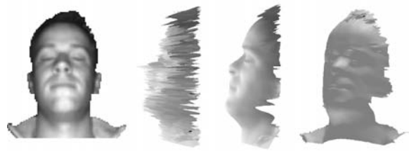
Figure 5: Improvement of range map quality using the shading constraint. From left: Intensity image; lateral view of raw measured surface; and surface reconstructed using the shading constraint in lateral and frontal views.
