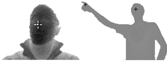
Figure 10: Left: Example nose-detection results shown on ToF range image; detection error rate is 0,03 [BHMB08a]. Right: The direction the user is pointing in can be computed from the difference vector between the positions of the head and hand [HBMB09].
