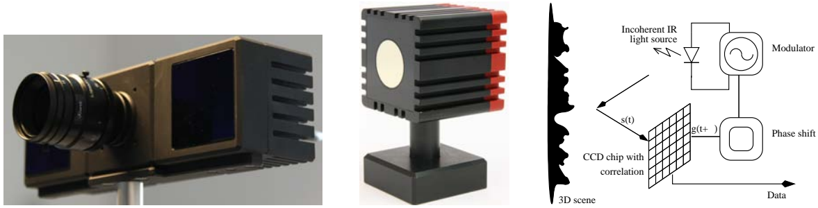
Figure 1: Left: PMDTec/ifm electronics CamCube sensor; Middle: MESA SR4000 sensor; Right: The ToF phase-measurement principle.
