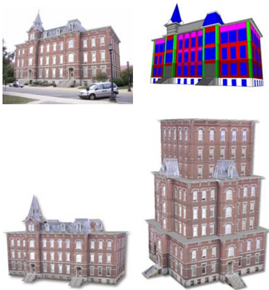
Figure 7: Style grammars for visualization of architecture [ARB07]. The user creates and subdivides an initial model of the building (top left). Repetitive patterns of the building features are automatically found and a representative grammar is constructed (top right). The user can then view the captured model (bottom left) and change the model on the fly producing new models (bottom right).
