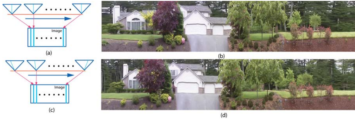
Figure 2: Pushbroom and Cross-slit Camera. (a) The stationary column sampling routine for synthesizing a pushbroom panorama (b). (c) The linearly varying column sampling routine for synthesizing a cross-slit panorama (d) (courtesy of Steve Seitz).
