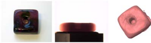
Figure 11: A photograph of a refractive object with absorptive properties (left), a tomographic projection obtained by matching the refractive index of a surrounding medium to the one of the object (middle) and the object's surface generated by iso-surface extraction on a volumetric representation of the absorption density of the object (right). The absorption density is reconstructed by tomographic means [TBH06].
