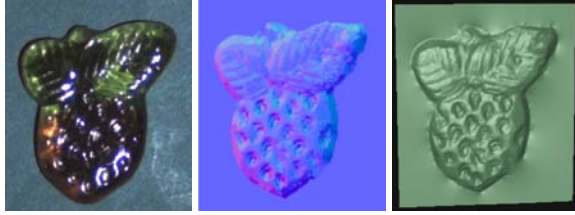
Figure 3: The photo of a jelly candy, exhibiting sub-surface scattering (left), a normal map acquired with the shape-from-specularity approach of Chen et al. [CGS06] (middle), and three-dimensional surface shape obtained by integrating the normal field. Image courtesy of Tongbo Chen, Michael Goesele and Hans-Peter Seidel.
