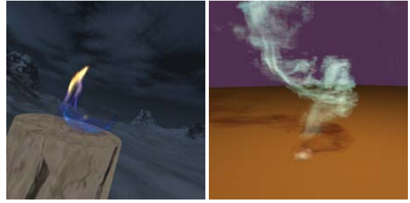
Figure 13: Results of tomographic reconstruction on fire [IM04] (left) and smoke data sets [IM05, IM06] (right). The multi-view setup used to capture the input data consists of 8 cameras, Reconstruction resolution is 128^3 (left) and an octree-representation with effective resolution of 256^3 (right).
