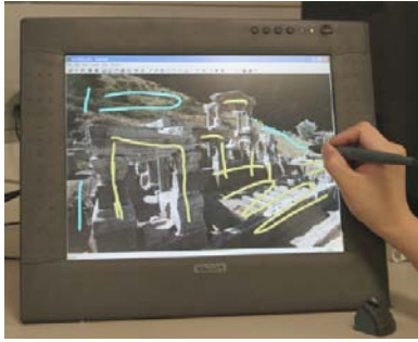
Figure 4: Input to a sketch-based system is acquired from pen-based or free-form devices such as a tablet display (reproduced from [YXN*05]).
