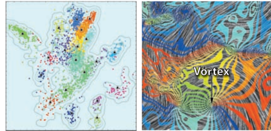
Figure 10: A layered combination of glyphs, color coding and isolines (left) and a filigreed layered visualization of flow data combining texture advection and color coding [WFK*02]. (Image courtesy of P. C. Wong)
