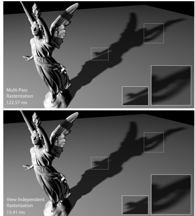
Figure 5: Multi-view soft shadows rendered using traditional multi-pass rasterization of polygons (top) compared to VIR paired with our parallel view rendering approach (bottom). Both methods produce 128 high resolution depth maps and similar high quality shadow penumbra, but VIR takes only a fraction of the time.
