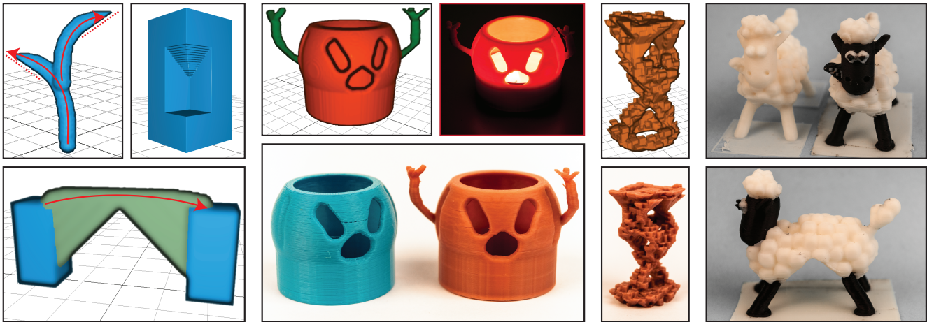
Figure 2: Left: examples of an add-trim stroke, a remove-preserve operation where a cube is subtracted from a pillar, and an add-grow stroke which automatically creates a bridge underneath. Center: the PUMPKIN model can be used as a tea-light holder. Center Right: a more intricate sculpture. Right: more prints of the SHAUN model. All shapes here print support-free.
