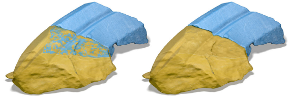
Figure 3: Left: Unconstrained registration yields mutual penetrations of the source and target contact surface, which might be undesirable in object reassembly applications. Right: Inclusion of constraints for non-penetrating registration. To better illustrate the mutual penetrations, the fragment in front is rendered with transparency.
