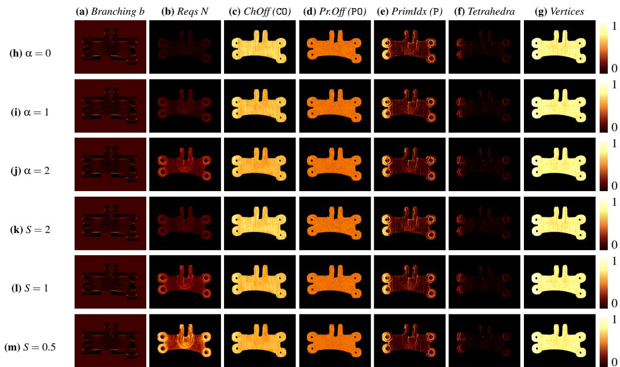
**Figure 4:** Analysis for rendering the SimJEB122 model visualizing the branching rate  $b_{(x,y)}$ , numbers of requests  $N_{(x,y)}$  normalized by  $2^{15}$ , and cache hit rates  $p_{(x,y,i)}$  for individual allocations  $i$ .
