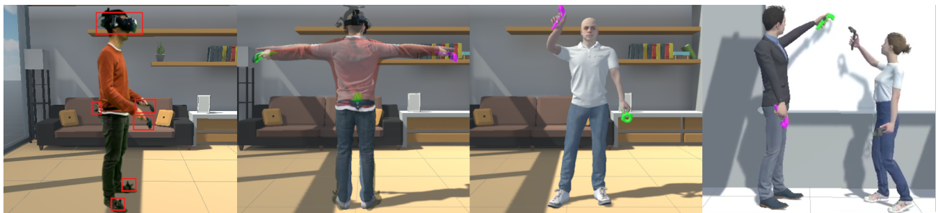
Figure 1: Set up for computing the exact offsets between the trackers and the avatar's joints to obtain a better match of poses and movement, using only one HMD, two controllers and three trackers.
