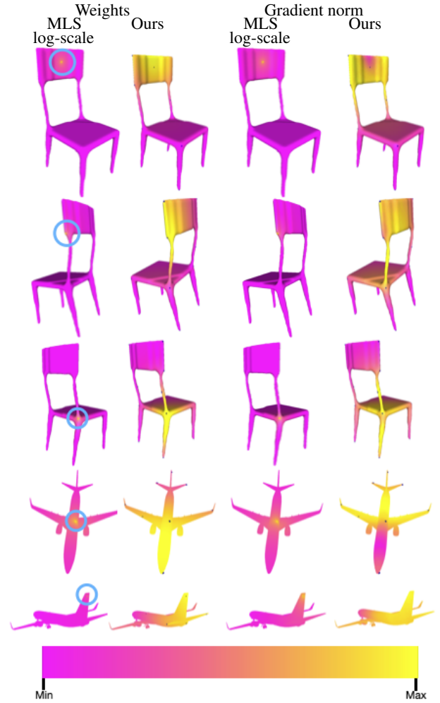
Figure 7: In this Figure, the weight function and its gradient norms are visualized as heat maps for the control points circled in blue at the leftmost column, with the MLS weights and gradient norms being in log-scale. This illustrates our method's ability to produce more piecewise smooth deformations compared to plain MLS, as our weight function is more evenly distributed over each control point adjacent region, where adjacent is with respect to the entire control point configuration, compared to the sharp peaks produced by plain MLS. This Figure also emphasises NeuralMLS's approximation characteristics compared to MLS that is an interpolation technique, as weights near control points are not very steep compared to their surroundings.
