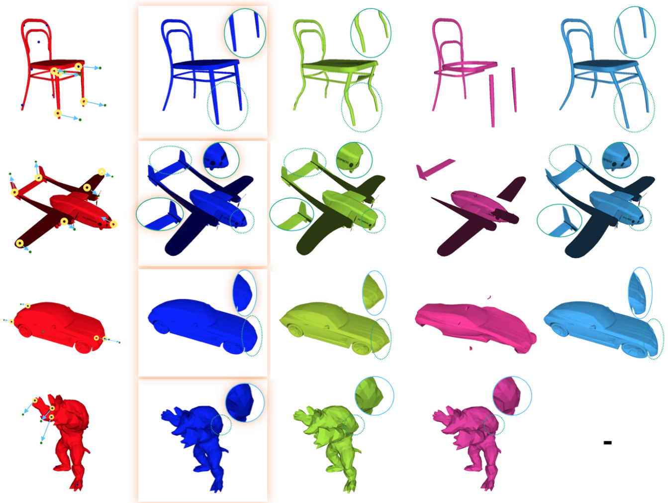
Figure 4: Comparison of our method to other control point based deformation methods. Our method achieves desirable results compared to traditional and learning-based deformation techniques. Note that the first three rows are non-manifold meshes, which ARAP does not support. Since KPD requires a dataset to be trained on, results for the "armadillo" shape (bottom row) cannot be obtained.
