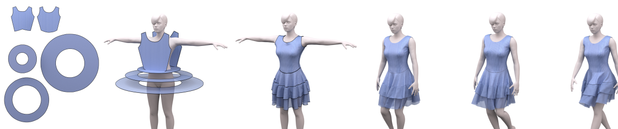
Figure 1: By using our tool, multiple layers of 2D patterns are placed around a virtual character and stitched together interactively.
