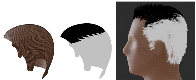
Figure 8: Segmenting the top of the scalp with a black&white texture. Hairs in the black area are defined as being in the top region.
