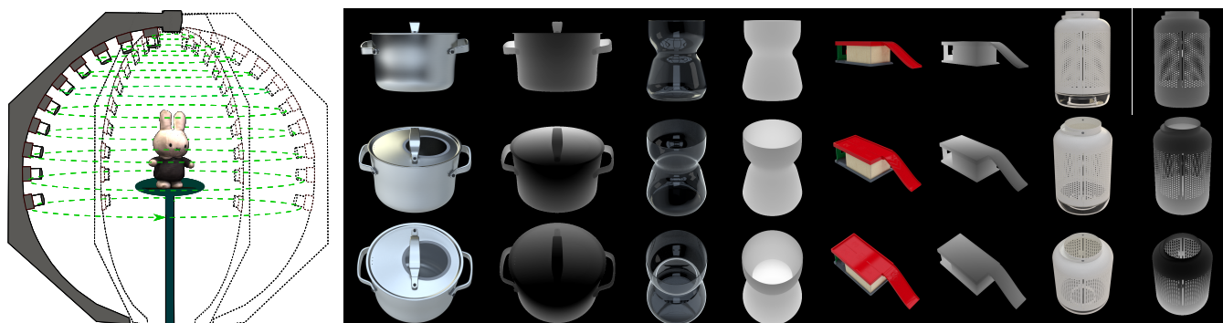
Figure 1: Left: schematic of our 360° inward-looking light field capturing system that consists of a precision guided rotating arm with multiple cameras. Right: a few samples of the synthesized light field images from different data sets and their corresponding depth maps.
