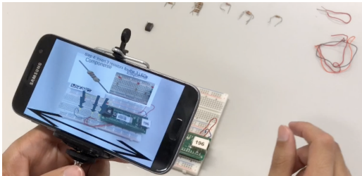
Figure 3: Condition 2- Circuit assembling using the AR single-device approach.
