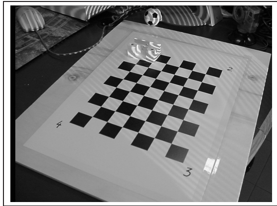
Figure 8: A digital image of a simple component with artificial fringes projected on it.
