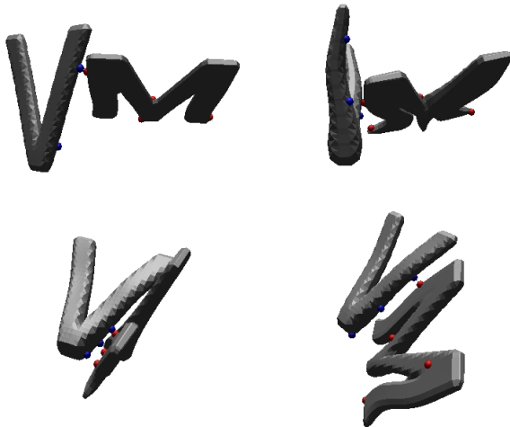
Figure 2: Illustration of collision detection between two models undergoing CSRBF deformations.
