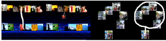
Figure 6: Relation Stroke. The user can create a layered layout by drawing relation strokes (left). Multiple nodes can be connected to one node at the same time (right).
