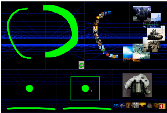
Figure 3: Normal Stroke. The user can control the information size by selecting the appropriate pen width (top) and adjusting the paint area (bottom). The preview rectangle shows how the information size is displayed within a painted area (bottom).
