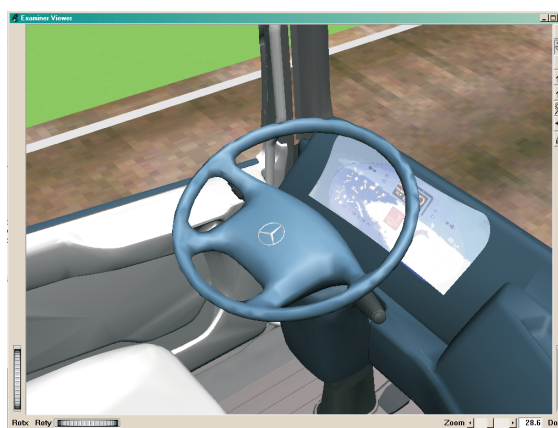
Figure 1: Simulation of reflections on instrument cover
