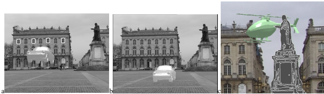
Figure 2: (a) Registration using only 2D/3D correspondences; (b) Registration with the mixing method (c) Occlusion resolution.
