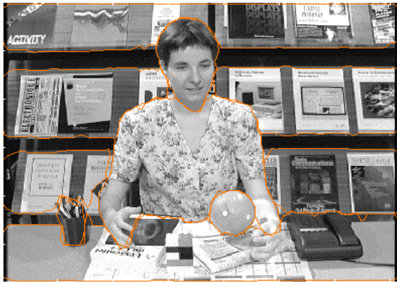
Figure 5. The final segmentation of the given point cloud into sub-surfaces. The borders of the surfaces determined by the algorithm match exactly to the actual objects' boundaries.
