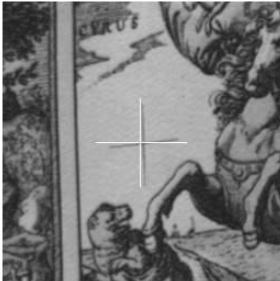
Figure 3: The repositioning accuracy over one of the monitored regions is shown by the superposition of the white crosses (image centers) to the dark crosses (test points)
