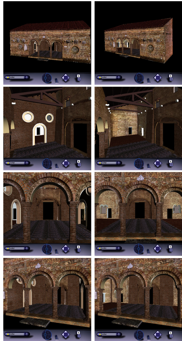
Figure 4: conservation project: interactive comparison between the VRML model of the present state (left) and the new configuration without buttresses (right).
