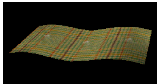
Fig. 8: Rendered view of the three lobe mode in Euler-Buckling.
