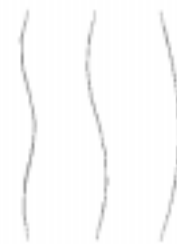
Fig. 7: Three modes of Euler-Buckling as simulated by our method.
