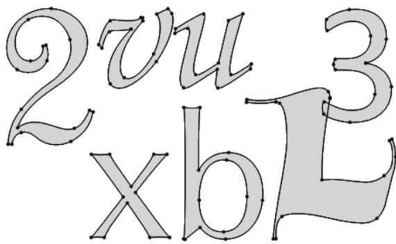
Figure 4: The computed salient points reliably indicate high curvature with little algorithmic tweaking and only two uncritical parameters (examples from well-known typefaces).
