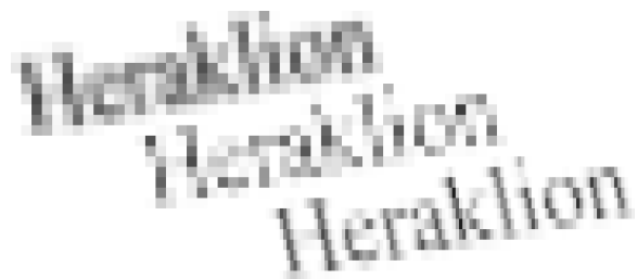
Figure 1: Standard texturing leads to excessive blur (top, strongly magnified). Negative MIP level bias (mid) and RGB subpixel rendering can help (bottom; this grayscale print does not reveal the detrimental color fringes).
