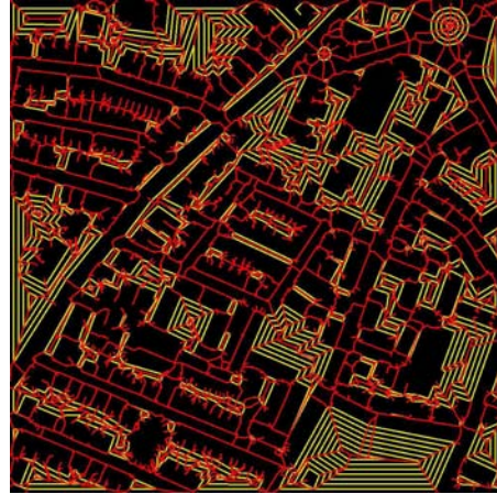
Figure 3: Iterative Shrinking Polygons: Straight skeleton in red, free space in black and iterative shrinking polygons in yellow.
